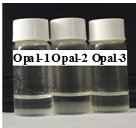
Fig. 2. Digital photo of the dispersion of the OPal samples prepared under different temperatures after standing for 30 min.
