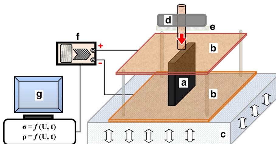
**Fig. 2.** The apparatus for direct measurement of resistivity and conductivity of pressed pellets. a: pressed tablet sample (oriented for measuring in direction perpendicular to the direction of pressing), b: polished Cu electrodes, c: flexible insulator, d: weights to ensure a constant pressure on the sample in the direction of the red arrow, e: felt muffler, f: DC source and measuring card, g: computer with software.
