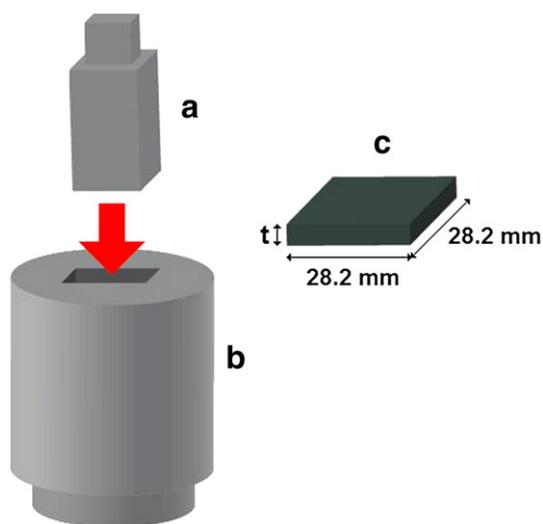
**Fig. 1.** a) Piston, b) matrix and c) pressed tablet. Thickness  $t$  varies in dependence on type and amount of composite.
