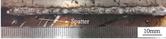
Fig. 1. Weld seam appearances of 5083 aluminum alloy (laser power 5 kw, welding speed 2 m/min).
