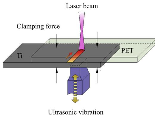
Fig. 1. A schematic diagram showing the U-LAMP method.
