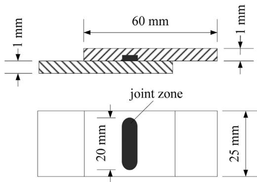
Fig. 2. The dimensions of the lap joint.
