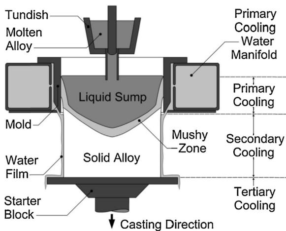
Fig. 1. DC casting setup and different components [reproduced from Baserinia et al. [9]].
