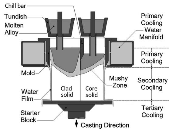
Fig. 2. Schematic of DC co-casting for multi alloy system.
