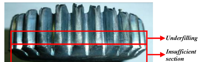
Fig. 3. Extruded gear with the insufficient section of gear face and the underfilling of gear tooth.
