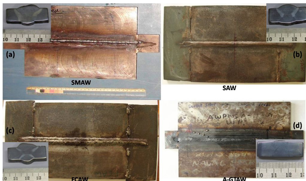
Fig. 1. Macrostructure photos of HSLA steel arc welded joints—SMAW, SAW, FCAW and A-GTAW.
