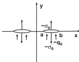
Fig. 1. Two collinear cracks embedded in an orthotropic solid under combined thermomechanical loadings.
