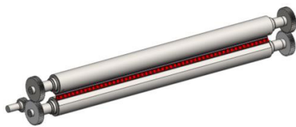
Fig. 1. Rotating transverse paper cutting machine simple structure.
