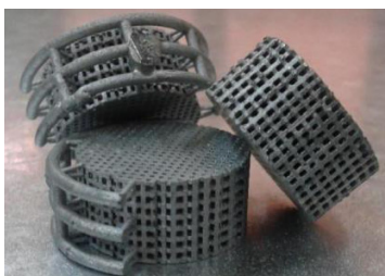
Fig. 1. Example of cylindrical metal foams obtained by investment casting.
