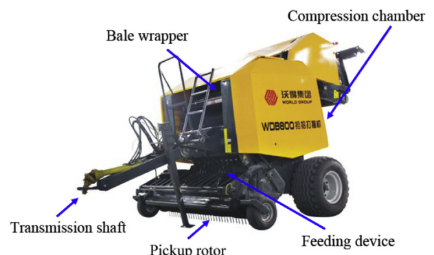
Fig. 1 – WDB800 steel-roll round baler.
