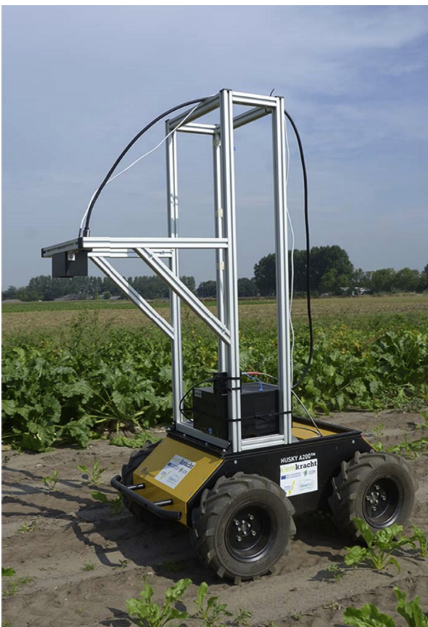
Fig. 1 – The robotic platform for volunteer potato control in a sugar beet field.
