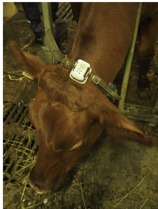
Fig. 1 – Ubisense tag attached to the collar of the cow.
