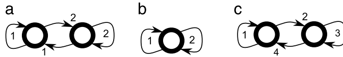
Fig. 1. Both automata on Fig. 1(a) and (b) accept arbitrary switching sequences on two modes. The third automaton (Fig. 1(c)) is on 4 modes. It does not generate arbitrary switching sequences, mode 1 must be followed by mode 1 or 2, mode 2 by mode 3 or 4, etc.
