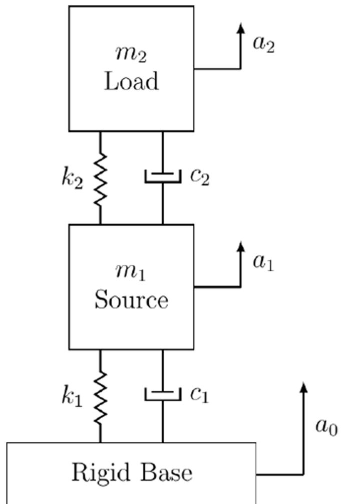
Fig. 2. Simple two DOF coupled system.
