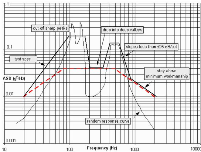
Fig. 1. Example Test Envelope Synthesis taken from Ref. [18]. The thin line is response curve and thick line is the test envelope created around it, with the dashed line representing minimum workmanship levels.
