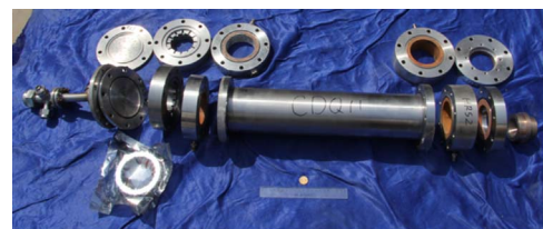
Fig. 1. Physical composition of hybrid rocket motor.
