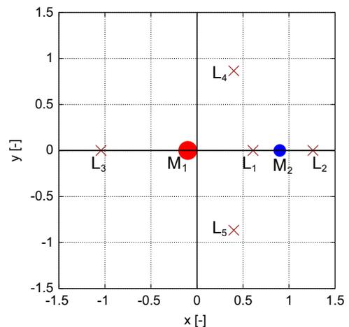
Fig. 1. The Lagrangian points,  $L_1, \dots, L_5$ , in the rotating frame.
