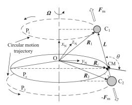
Fig. 1. Scenario of internal forces connected two spacecraft formation with unequal masses.
