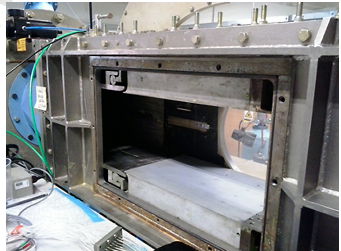
Fig. 1. Transonic wind tunnel with side door removed; flow direction right to left.
