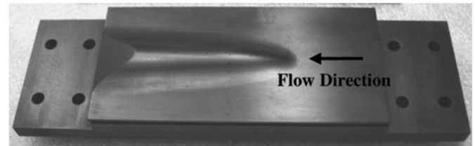
Fig. 2. Three-dimensional view and photograph of the Boeing Bump-compression surface [21].
