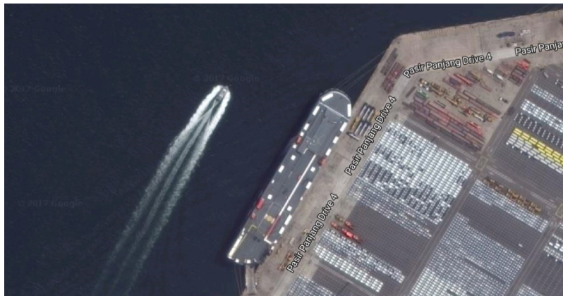
Fig. 1. The wash waves produced by an advancing ship. (Google Map. https://www.google.co.uk/maps/@1.2841423,103.7517161,382m/data=!3m1!1e3?hl=zh-CN ).
