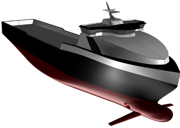
Fig. 1. The case vessel with wavefoils deployed.
