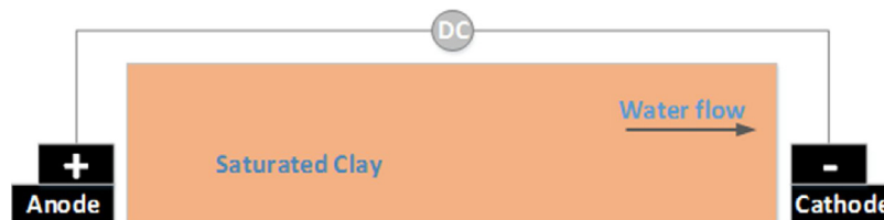
Fig. 1. Electro-kinetic phenomena: electro-osmosis.
