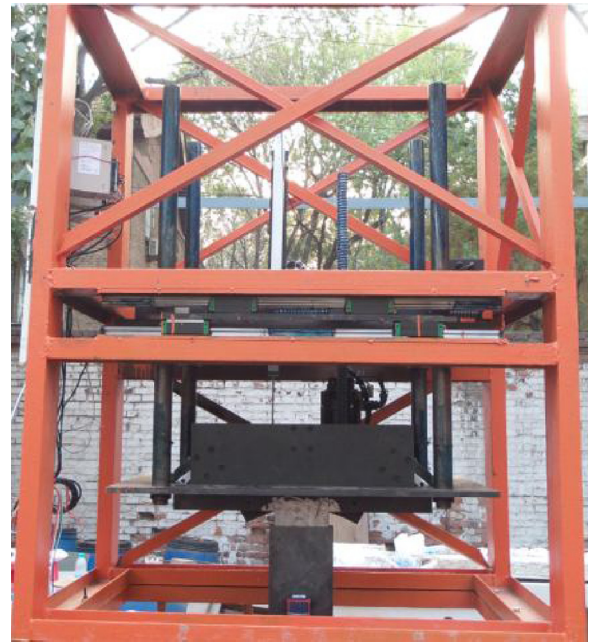
Fig. 2. Three-degree-of-freedom loading rig.
