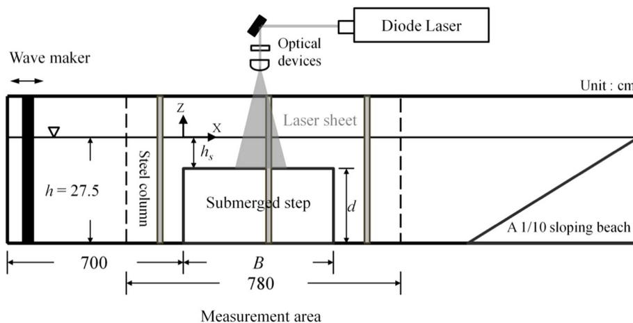
Fig. 1. Wave flume and experimental setup.
