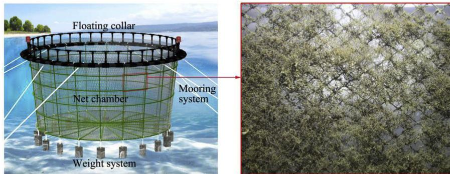
Fig. 1. Sketch of the net cage (left) and biofouled net (right).
