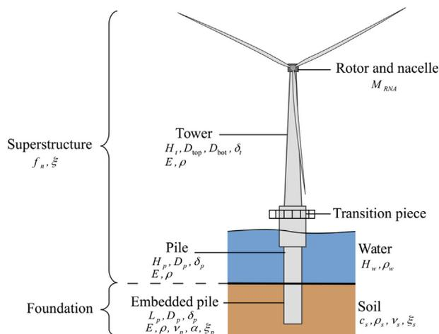
Fig. 1. Representation of a generic OWT and identification of geometrical and material parameters.
