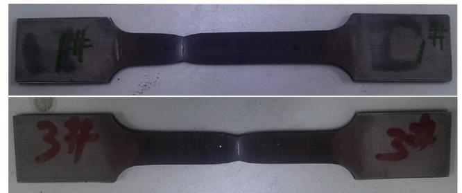
Fig. 2. Photo of specimens fractures at different position. The upper half is specimen of the RD group, and the lower half is specimen of the other group.
