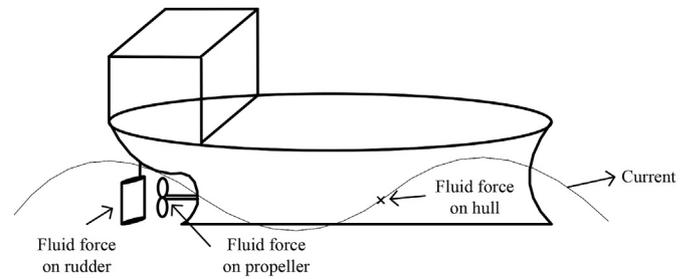
Fig. 1. The fluid force affecting on different parts of a vessel.
