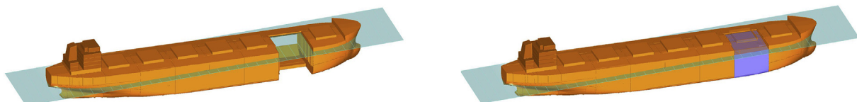
Fig. 2. 3D visualization of the lost buoyancy (left) and the added weight (right) methods.
