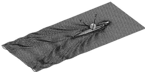
Fig. 2. The coordinate system and panel distribution on the computational domain of a Wigley III hull advancing in open calm water. There are 9900 panels distributed on the half computational domain: 300 on the body surface and 9600 on the free surface. The computational domain is truncated at L upstream and 2L downstream. The figure also shows the waves produced by Wigley hull at F_n = 0.3 , where F_n = u/\sqrt{gL} is the Froude number.
