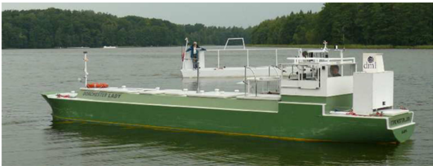
Fig. 4. The ship “Dorchester Lady” on the lake Silm (in the front). The floating model of the passenger ferry “Stena Germanica” is seen at the back.
