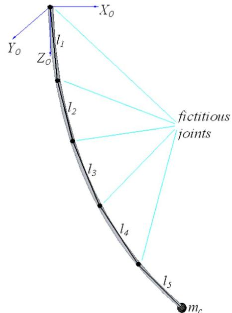
Fig. 2. Continuous flexibility and its discrete approximation.
