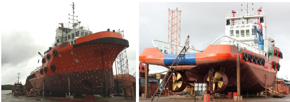
Fig. 1. As-built 40 m anchor handling tug (AHT).
