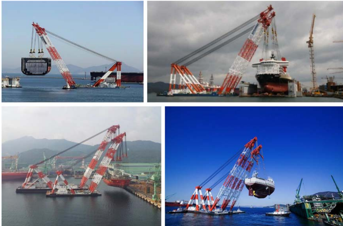
Fig. 1. Typical examples of block lifting by using floating cranes in shipbuilding production.
