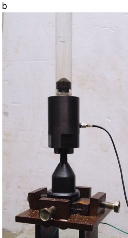
Fig. 1. Structure of experiment device. (a) Diagram of the experiment system. 1. Observation chamber, 2. sprayer, 3. seal film, 4. combustor, 5. pressure hole, 6. pressure sensor, 7. charge and 8. ignition electrodes. (b) Picture of the multigas jets device.
