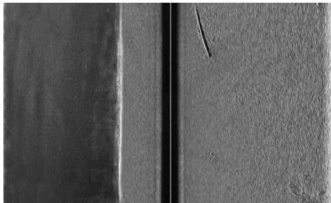
Fig. 2. Side-scan sonar track recorded by a towfish fixed to the vessel, positioned on the starboard side (the reflection of the hull is visible).
