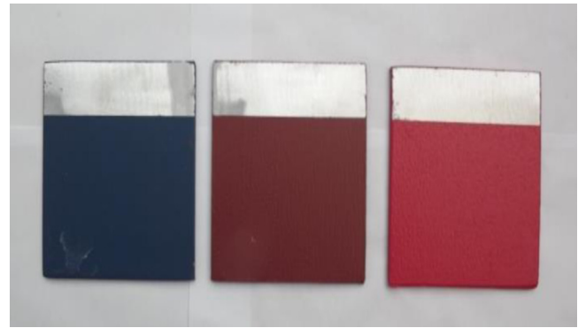
Fig. 2. Laboratory plates before immersion. (Left SPC, middle CDP and right AF).
