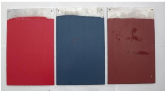
Fig. 1. Sea plates before immersion. (Left AF, middle SPC and right CDP).
