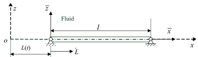
Fig. 1. The beam attached to axially moving supports immersed in fluid.
