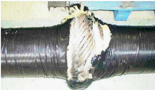
Fig. 2. Birdcaging failure ( Bectarte and Coutarel, 2004 ).
