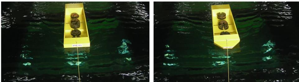
**Fig. 1.** Experimental barge model KNU-001 (left) and KNU-002 (right).
