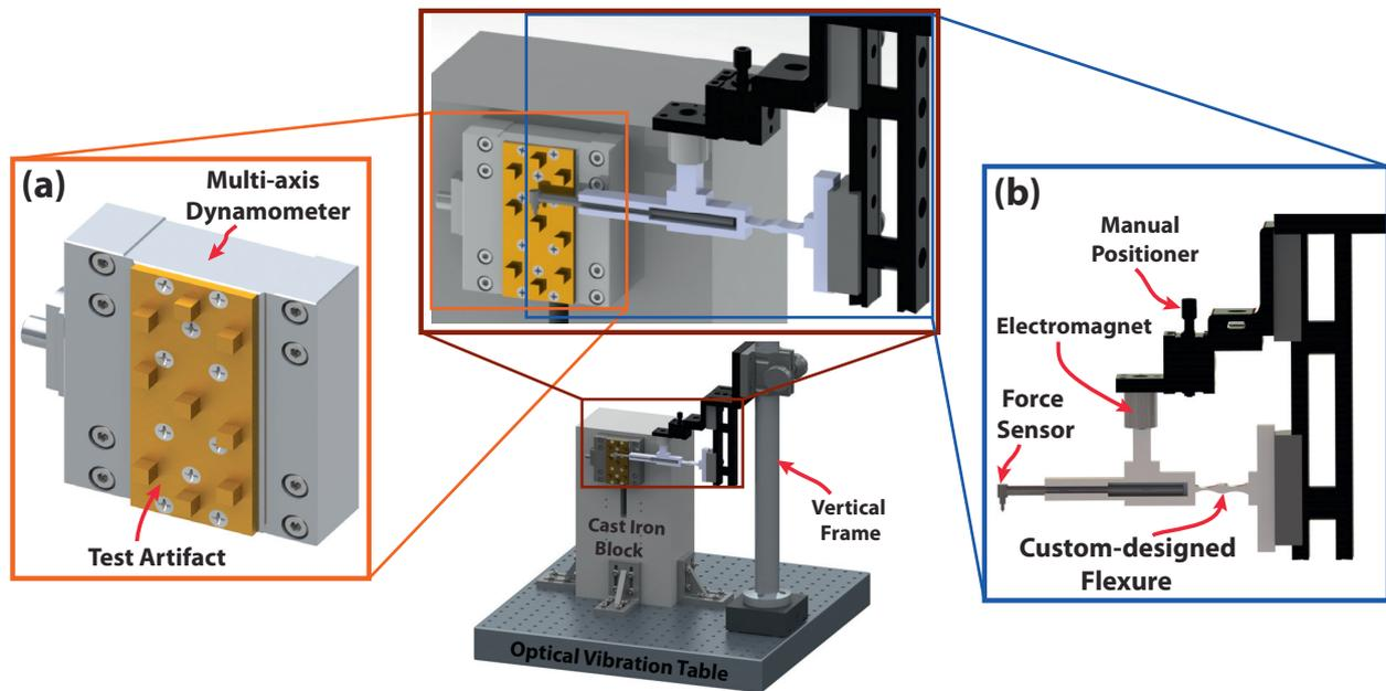
**Fig. 1.** The testbed for determination of 3D dynamic force measurement characteristics of multi-axis dynamometers: (a) the dynamometer with the attached test artifact; and (b) the impact excitation system to provide repeatable excitations within a broad range of frequencies.
