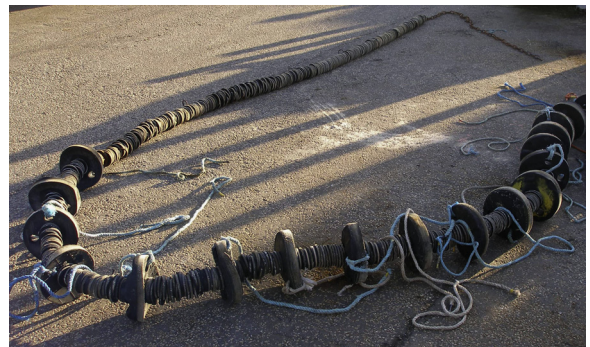
Fig. 2. Typical rock hoppers for a bottom trawl-net (Crown Copyright and reproduced with the permission of Marine Scotland Science).
