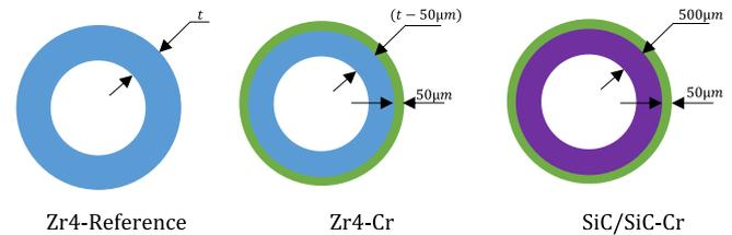
Fig. 1. Different Zr4-based claddings and proposed coating thicknesses.
