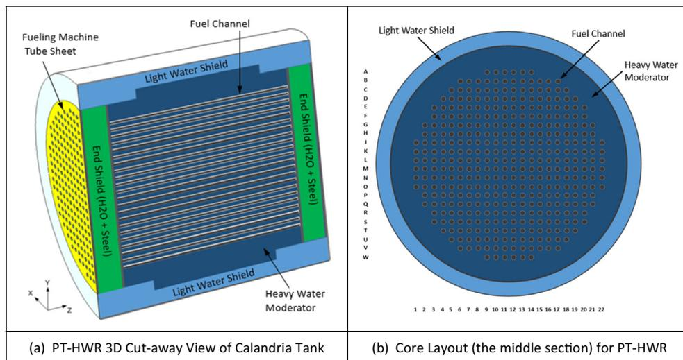
**Fig. 1.** Illustration of a Pressure Tube Heavy Water Reactor.
