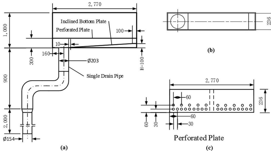
Fig. 1. The schematic of test section (a. Front view of the test section; b. Top view of the test section; c. Distribution of water entrance holes on the perforated plate).
