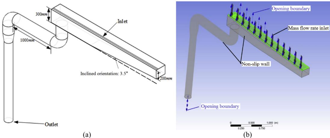
Fig. 2. The computational domain (a) and boundary conditions (b).
