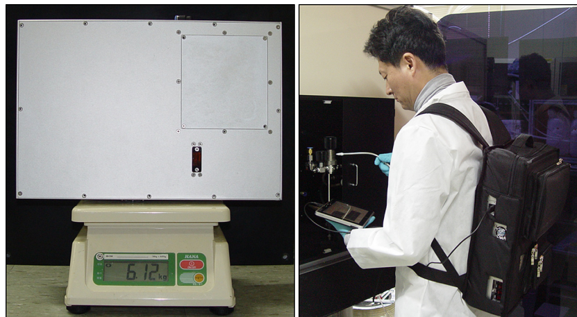
Fig. 1. The developed portable leak sensor body (left) and picture of searching for the leak point with the sensor (right).
