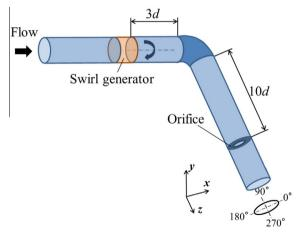
Fig. 3. Details of experimental test section.
