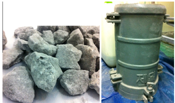
Fig. 2. Image of concrete rubble ( D > 50 mm) and mold ( D 15 cm \times H 30 cm) for scale-up test.
