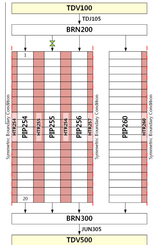
Fig. 3. RELAP5 nodalization map of SFE for single channel blockage transient simulation.
